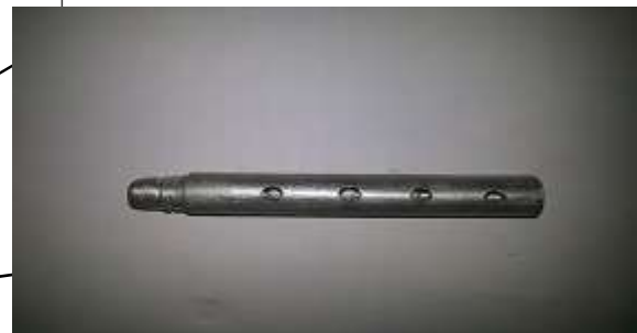
Fig. 6 Perforated Pin Fin used for the purpose
