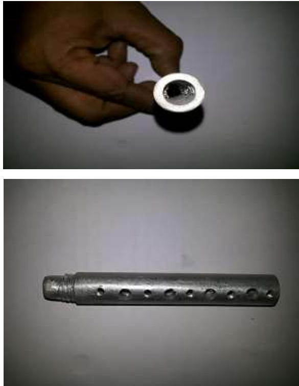
Fig. 7 Fin with four perforations used for the purpose
